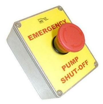
The ES1 switch is designed to fulfill the NFPA code requirements. It uses a heavy <u>cast aluminum</u>, weather sealed, NEMA 4X enclosure with stainless steel hardware. The switch is a large (40mm) red, single or double pole, 10 amp normally closed unit. The ES1 has a highly visible, bright yellow sign on the front panel for easy identification in an emergency. All components of the ES1 are UL listed.
